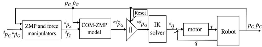
**Fig.3** Previous serial system structure with COM-ZMP model and bounding of integrator
