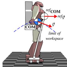
**Fig.1** Mismatch between robot and COM-ZMP model, with model and robot velocities,  ${}^{ref}v$  and  $v$ , respectively.
