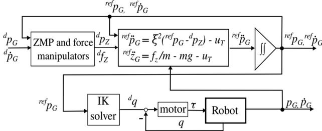
**Fig.4** Proposed parallel system structure with COM-ZMP model and virtual leader follower.
