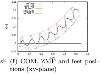
**Fig.6** COM reference, position, ZMP and knee angles profile for forward walking
