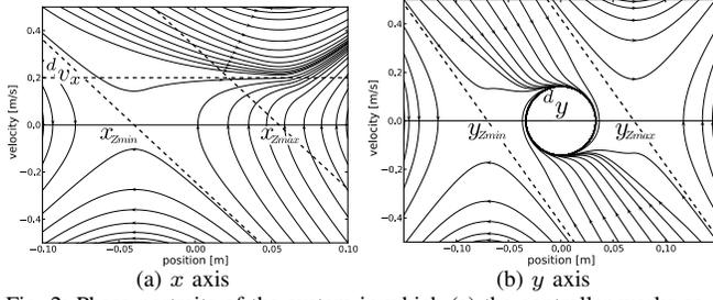
Fig. 2: Phase portraits of the system in which (a) the controller works as a velocity follower and (b) a stable limit cycle emerges
