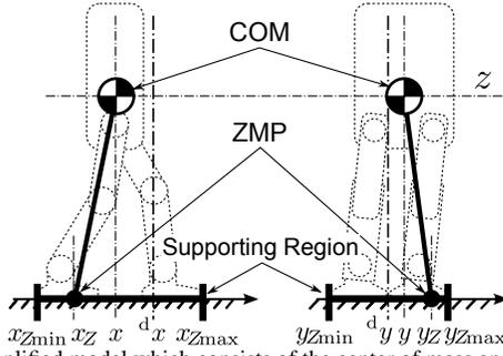
Fig. 1: Simplified model which consists of the center of mass and the ground reaction force distributed on a horizontal plane
