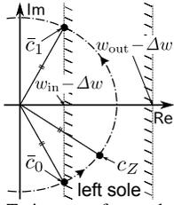
Fig. 6: Trajectory of  $c_Z$  when ZMP comes into and goes out of the sole
