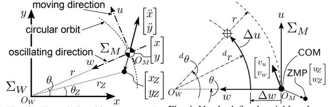
Fig. 3: The relationship between the fixed and moving frames
