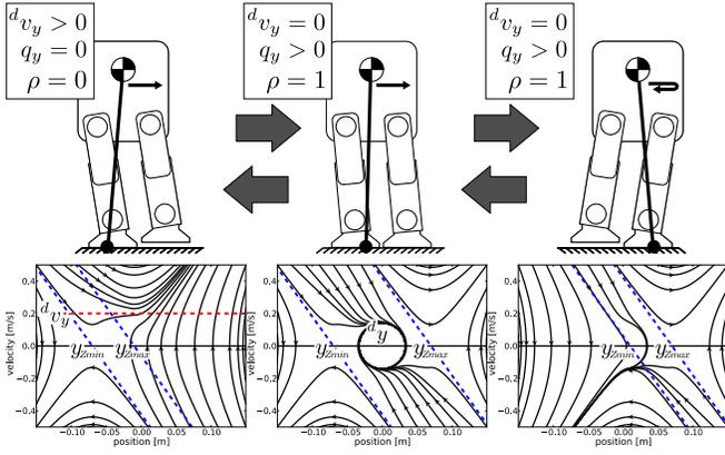
Fig. 6. Dynamics morphing along  $y$  axis with a desired velocity
