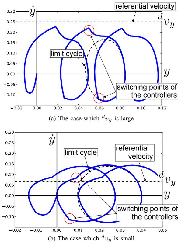
Fig. 9. Loci of COM in sideway locomotion
