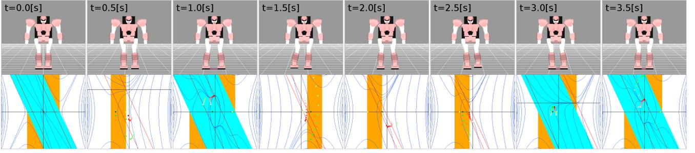
Fig. 7. Snapshots of the simulated sideward locomotion. The robot succeeded to continue walking with respect to  ${}^d v_y$  changed at random during the motion.
